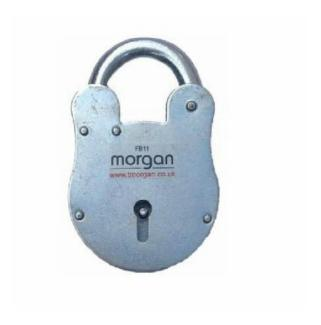
65mm padlock to pass London Fire Brigade FB11 key 10mm diameter steel shackle Maximum shackle clearance 18mm vertical x 25mm horizontal Zinc plated finish Also available with fitted 500mm steel chain - FB11C
